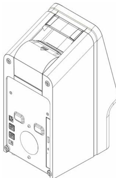
7. Place a clean filter flat in the fan vent. Tuck the sides of the filter underneath the vent's edges.
