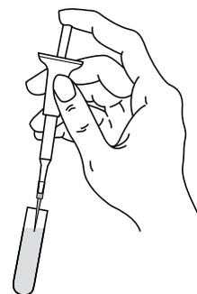
4. *Slowly* release the plunger to draw the sample. Pause, then remove the pipette from the sample tube.
