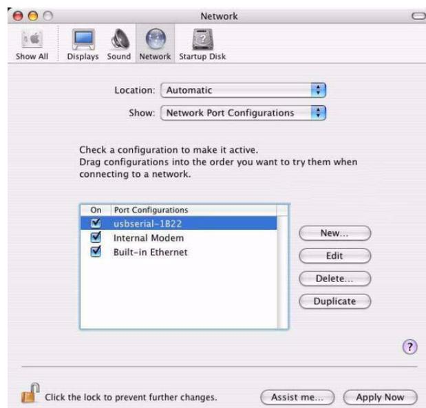
10. Configure any needed applications to communicate with the analyzer over the virtual communication port.
